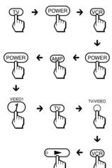
You can program up to 16 consecutive steps on each of the SYSTEM CONTROL buttons (A – D), including the initial step of pressing switch to a Component Select button.
