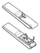
Insert the batteries (negative end first) through the guide clamp within each compartment as shown above.
