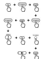
You can program up to 16 consecutive steps on each of the Component Select buttons, including the first step of pressing to select a Component Select button.
