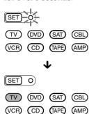
When erasing of a "learned" function is completed, the SET indicator light turns off.
