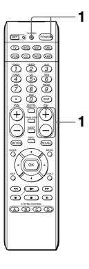
**1** Press and while holding POWER, press TV/VIDEO and CH +.
